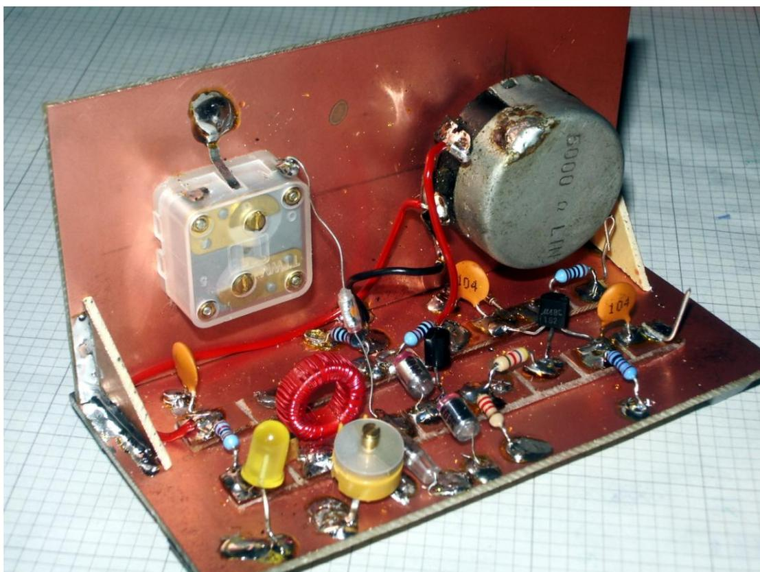
**Photo 5 - Rear view of completed VFO with front panel fitted.**
