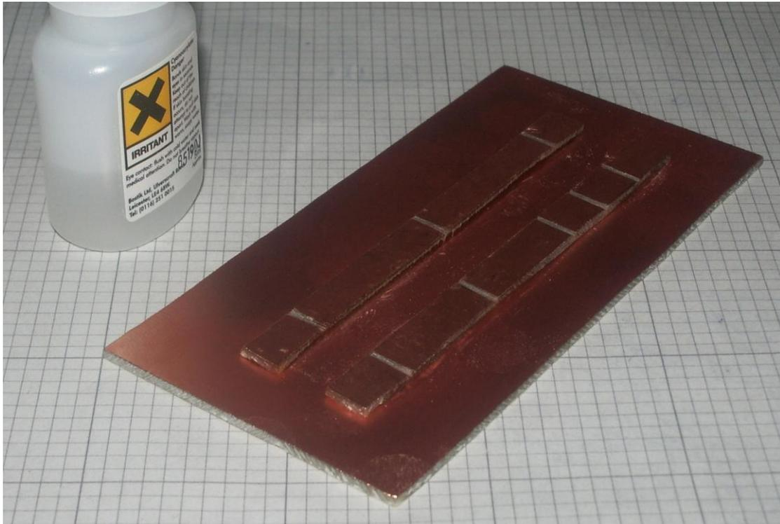
**Photo 1 - PCB 'Base' with island strips glued in place.**
